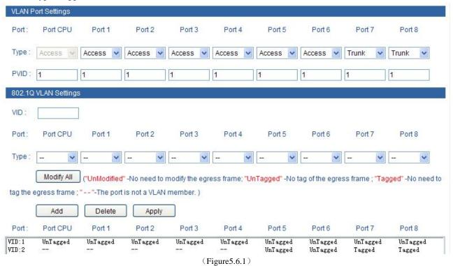
We can know as the figure, the type of port 7, 8 is Trunk, can allow the data of VLAN 1 and VLAN 2 pass.
